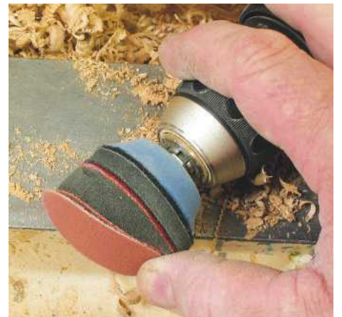
▲ Pic.15 Sanding a shape like this is fairly easy by hand, but Les prefers to power sand wherever possible so has attached a Simon Hope interface pad onto his arbor for flexibility
